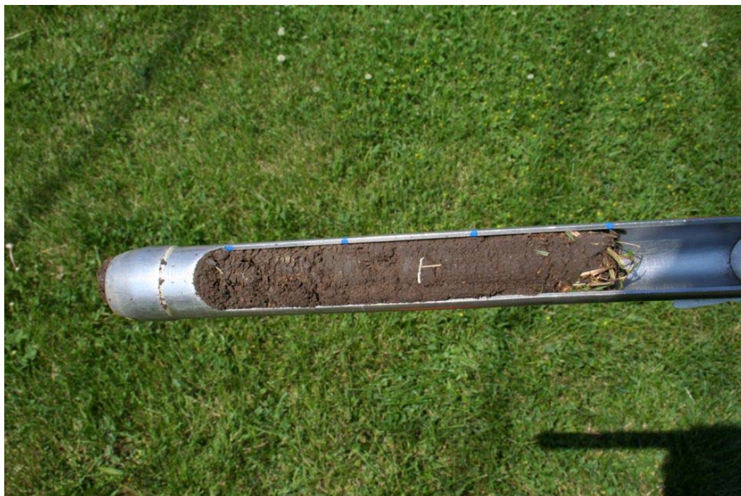
Photo 2: Typical core of soil to a depth of 20 cm. Photograph by M. Dixon, 12 June, 2013
